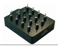
This multi channel pressure module is typically used for aerodynamic development, whereby pressure tappings can be made across surfaces of wings and aero features over the vehicle.
